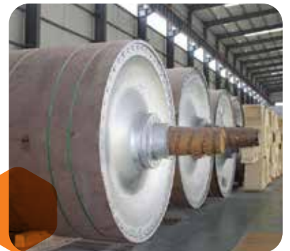
Dryer Drums are under machining of Paper Mill
