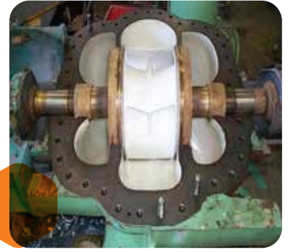
Complete Pump Rebuilding with Ceramic Coating
